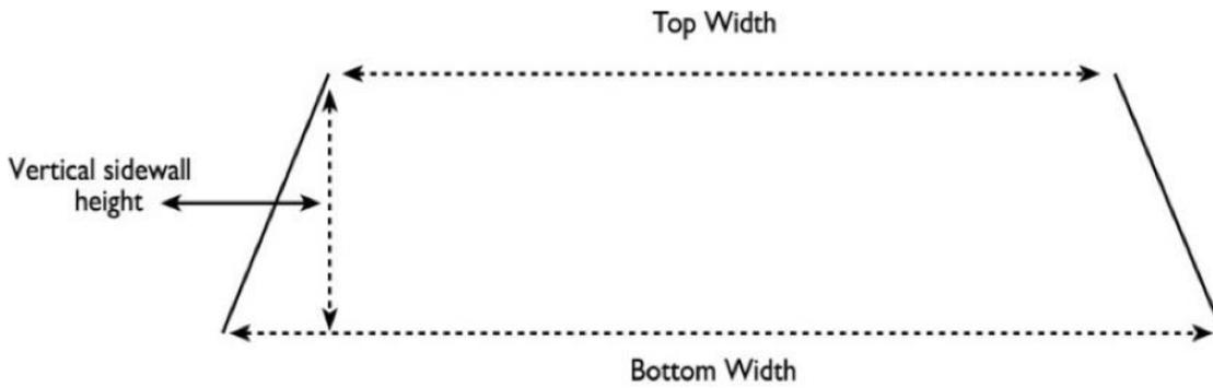
$$\frac{\text{Bottom Width} - \text{Top Width}}{\text{Vertical Sidewall Height}} = < 0.65\text{cm}$$
